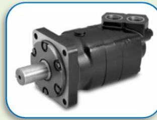
11-b. Four-bolt flange, Port choices. Keyed and spline shafts.
