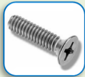
25 Knife section bolts, flat head counter sunk, stainless (1/4" UNC x 1/2" / 3/4" / 1" long)
