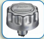
35 Screw-in filler breathers with 3/8" / 1/2" / 3/4" / 1" NPT male thread
