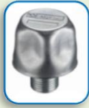
35 Screw-in filler breathers with 3/8" / 1/2" / 3/4" / 1" NPT male thread
