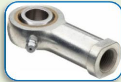
8 Female Rod end bearing with grease zerk. Sizes: 1/4" / 3/8" / 1/2" / 5/8" (Standard plated or stainless steel)
