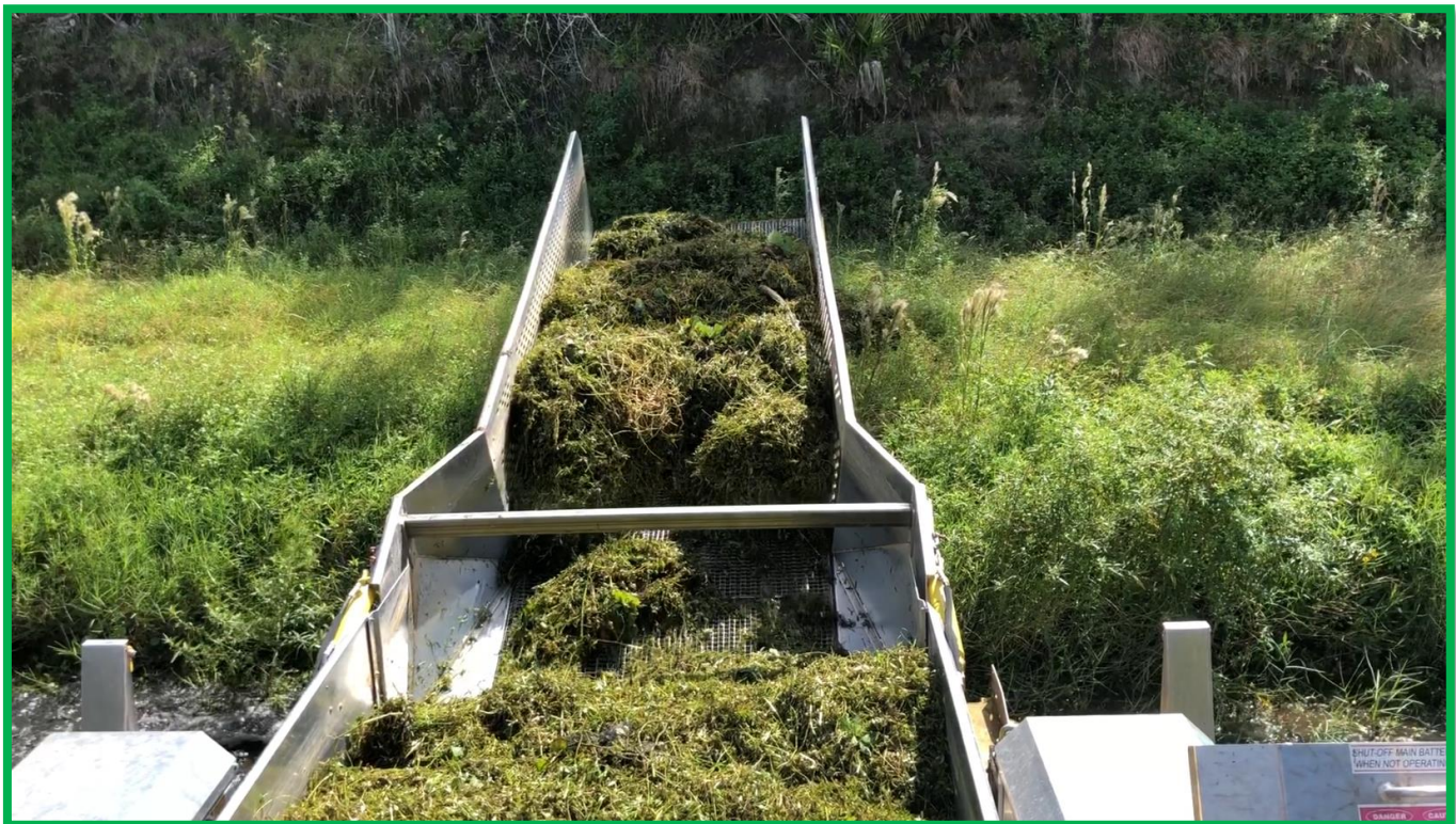
Unloading conveyor with 2.60 m / 8.5 feet long reach beyond the stern on all models. Discharge height hydraulically adjustable from horizontal to maximum of 1.5 -2.0 m / 5'-6.5 feet above water level. (varies with load size and placement)
