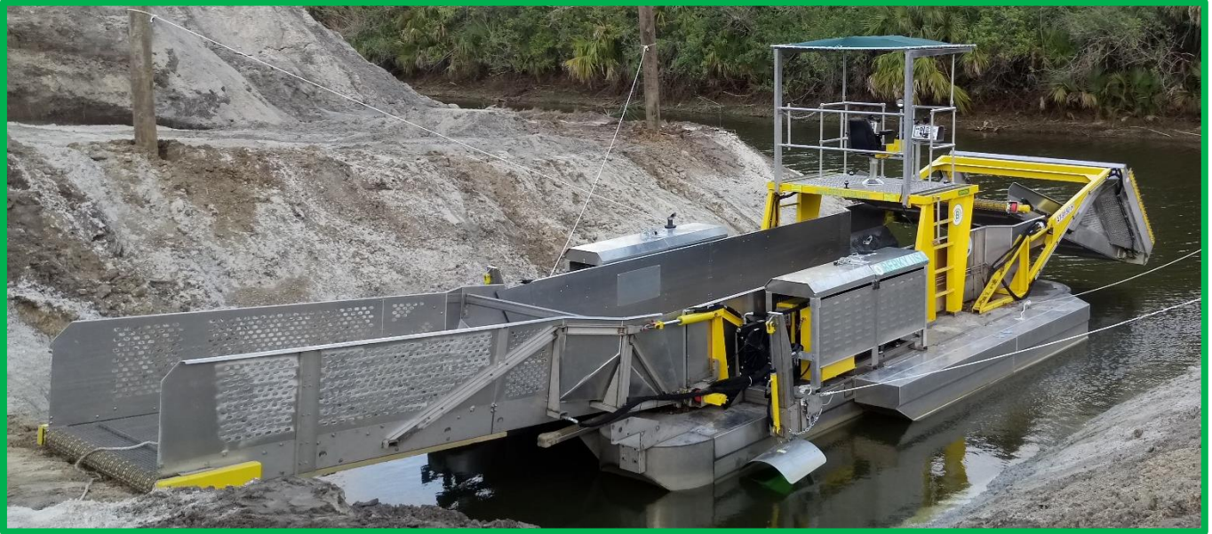
Modern Diesel/hydraulic power system. Hydraulic stern & side (shown) propellers
