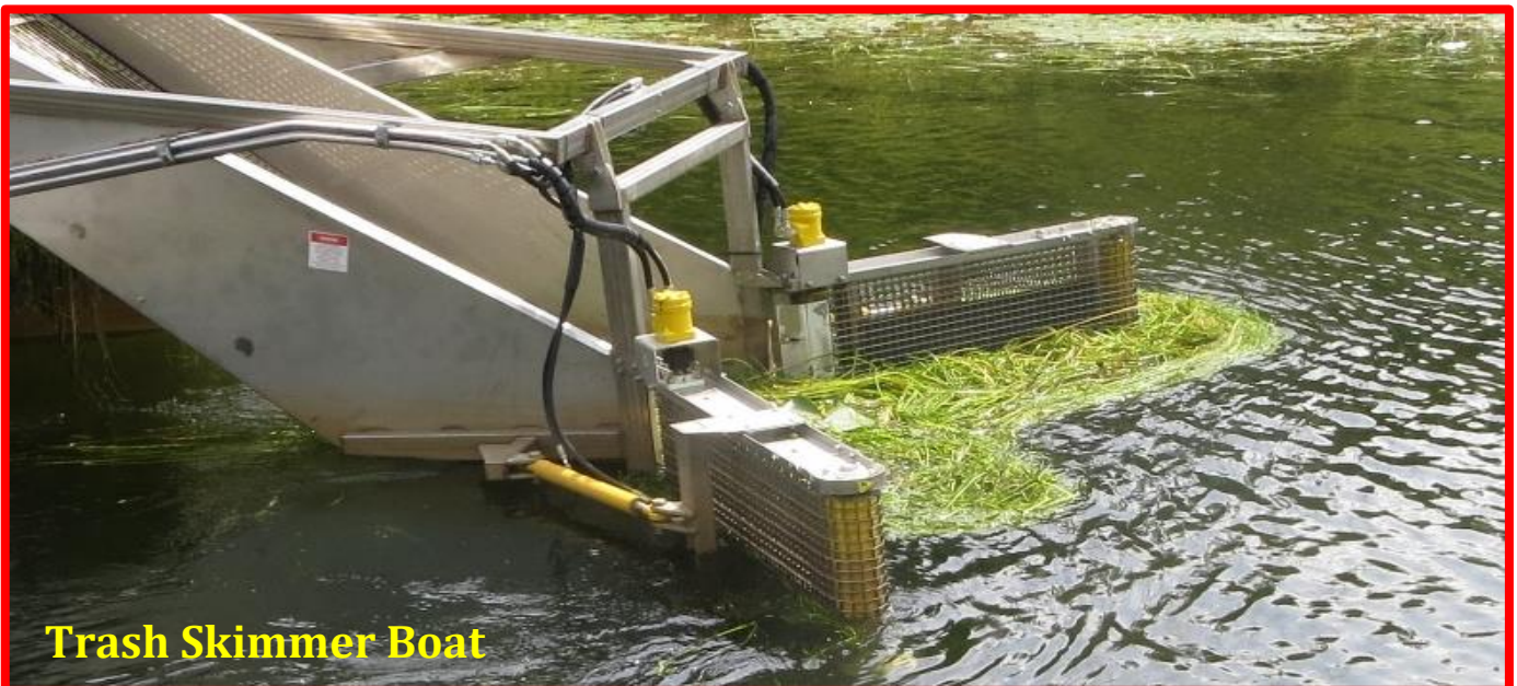
S12 S16 with side delivering skimmer heads. Conveyor wings can swing to maximum opening and completely or partially close to "grab" trapped objects . Use this head for floating weeds & trash, harbor and marina clean up. Sweep capacity from 3.65 & 5.00 m / 12 & 16 Ft. wide.
